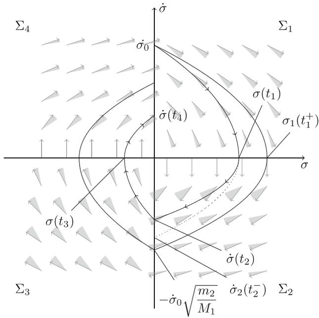
**Fig. 1.** Illustration of [Theorem 1](#). The arrowed curve represents a possible trajectory and the solid curve the majorant curve. The dotted curve bounds any trajectory from the initial condition  $(\sigma(t_1), 0)$ . The cones represent the set vector field obtained with the differential inclusion (9), and the black arrows the vector field that provides the majorant curve.
