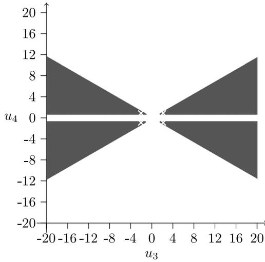
**Fig. 3.** Sets of  $(u_3, u_4)$  values that ensure establishment of 2-SM resulting from the conditions of [Theorem 1](#). The white crosses represent the values used for simulation.
